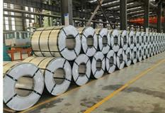
Due to the chemical activity of zinc is stronger than that of steel, even if there are small defects on the surface of the zinc coating, it can protect the steel substrate exposed on the surface after the zinc coating is missing
